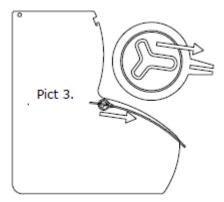
Replace the lid in the bin with the longest of the alignment pegs pointing upward. See picture 3.
